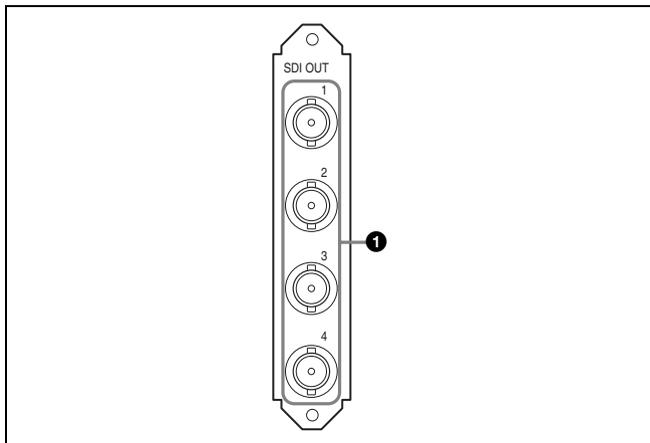
**① SDI OUT 1, 2, 3, 4 (3G/HD serial digital interface output 1-4) connectors (BNC-type)**
