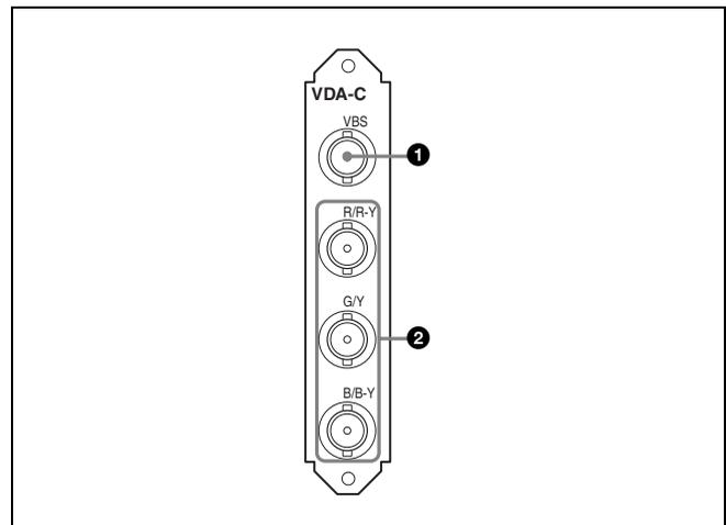
**❶ VBS (composite video signal output) connector (BNC-type)**
