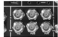
Component input video signals are A/D (input) converted (10-bit).
