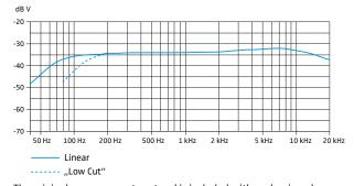
The original measurement protocol is included with each microphone, measured from 50 to 20,000 Hz.
