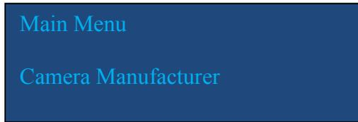
If the NAV button is pressed once the Camera manufacture menu can be seen. By tipping the NAV button up and down different manufactures can be chosen and if the relevant license has been obtained, selected. When the desired manufacturer has been reached, the NAV button is pressed once to select. The display will revert back to the Manufacture Status
