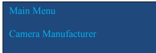
If the NAV button is pressed once the Camera manufacture menu can be seen. By tipping the NAV button up and down different manufactures can be chosen and if the relevant license has been obtained, selected. When the desired manufacturer has been reached, the NAV button is pressed once to select. The display will revert back to the Manufacture Status
