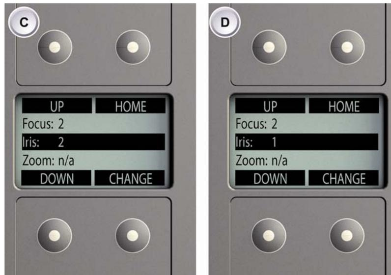
5. With **UP** or **DOWN** (C), select iris, focus or zoom motor (**n/a** means: motor not connected).
