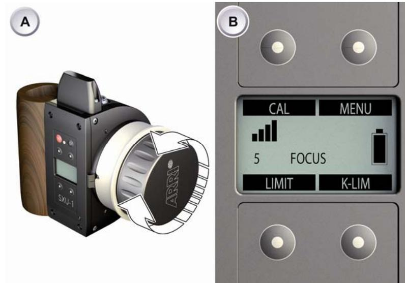
1. With control knob (A), turn lens axis to desired start position.
