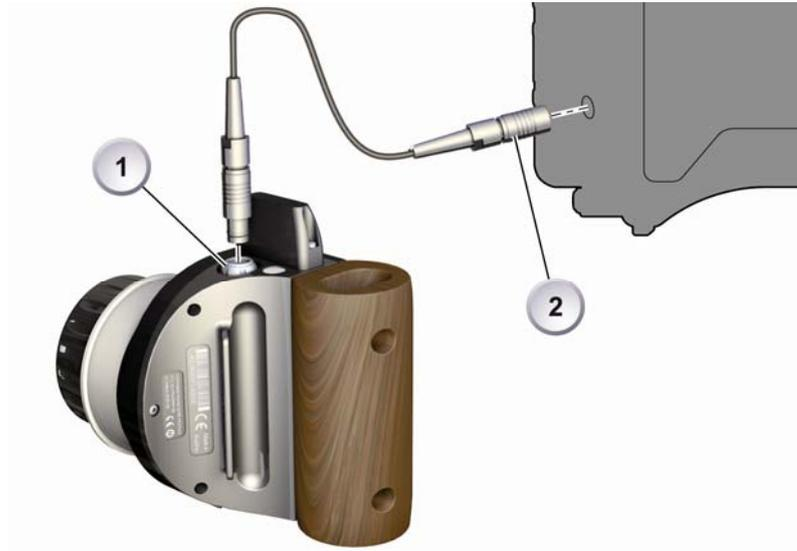
1. Connect product (1) to camera (2) via a standard LCS cable (maximum length: 75 m/250 ft).
