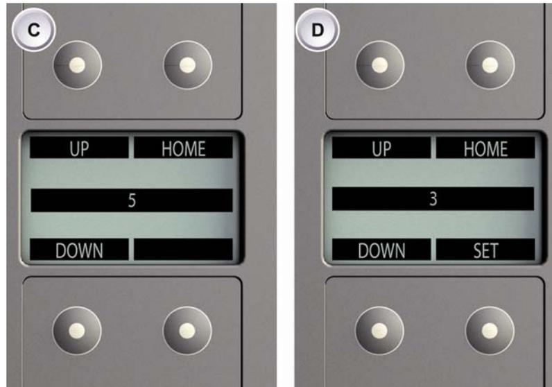
4. Submenu opens (C) on preset channel (*in this case: 5*).
