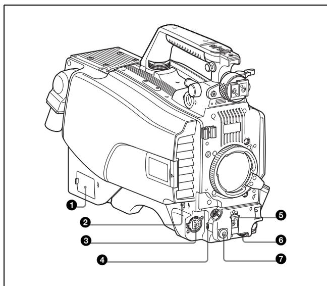
**1 NETWORK TRUNK connector (RJ-45 8-pin)**
