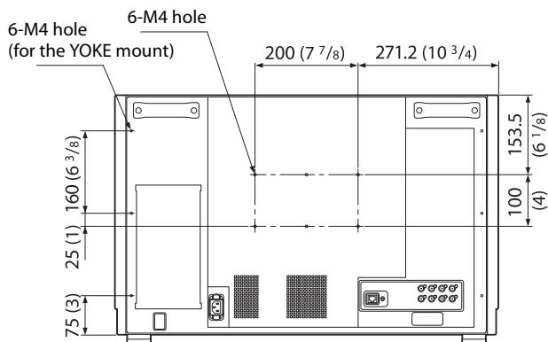
To install on a vehicle, fix the unit using screw holes for the YOKE mount.
